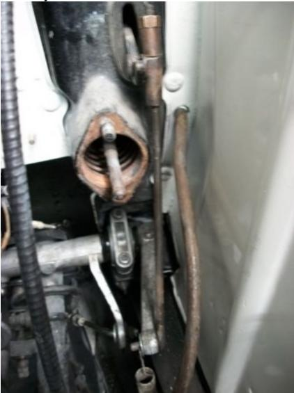
The first thing to do is to remove the support spring located at the bottom of this rod. Note that it is enough to simply unclip it from the bodywork side.
