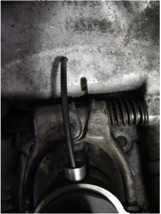
Once the clutch is assembled, one only needs to adjust the clutch set screw or guard; This guard setting is often poorly performed, and directly influences the longevity of the clutch release bearing (sometimes less than 10000kms)
