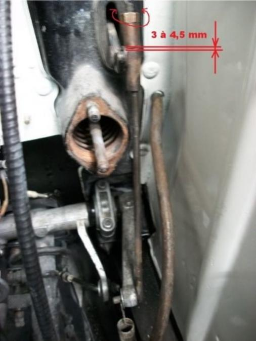
Once the actual setting of the clutch guard screw has been carried out, one only needs to replace the spring by re-hooking to body work.
