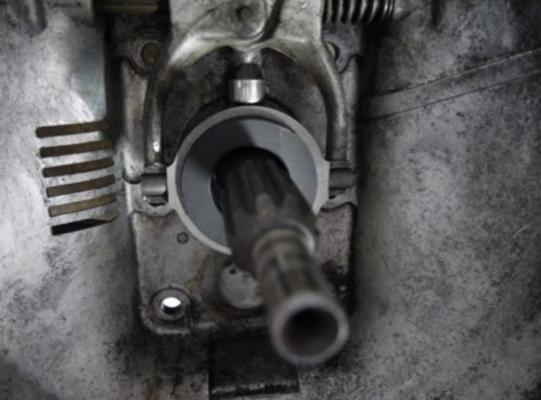
The the clutch release bearing studs will be mounted in this direction
