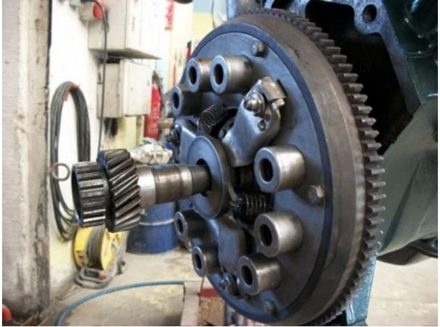
On the motor side the disc and the mechanism are mounted (centerer removed)
